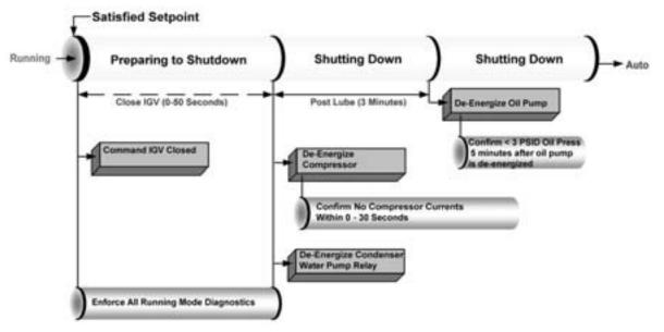
Figure 11. CVHE, CVHF and CVHG sequence of operation: normal shutdown to stopped and run inhibit
